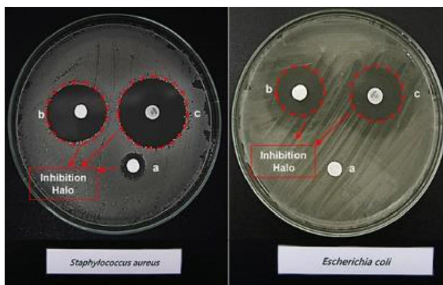
Figure 6. Antimicrobial activity against Staphylococcus aureus and Escherichia coli : (a) NRL biomembrane; (b) NRL-GS biomembrane and (c) Cellulose disc containing GS.
