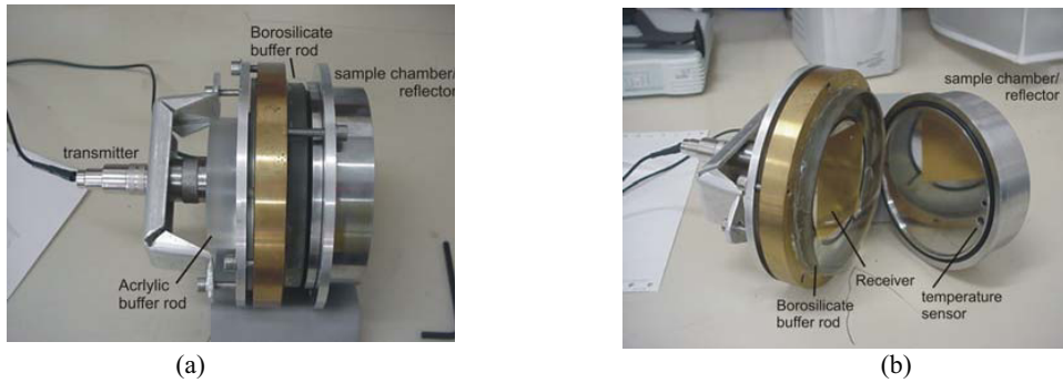
Fig.2 Density measurement cell: DET and sample chamber/reflector.
