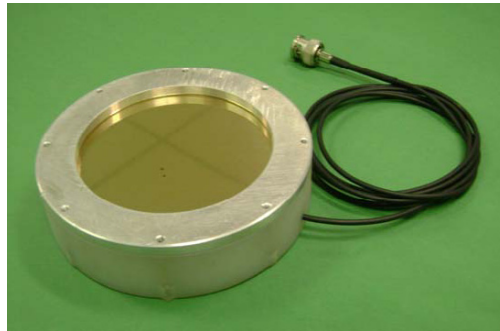
Fig.5 Large-aperture PVDF receiver.
