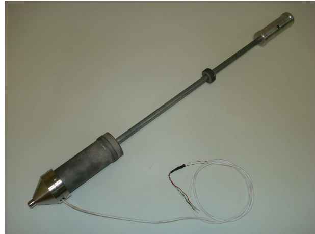
Figure 5: Details of new generation Portable Hardness Tester in wood with accelerometers
