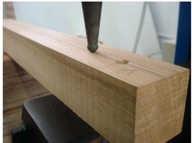
Figure 2: Details of indentation promoted by the Portable Hardness Tester in wood.
