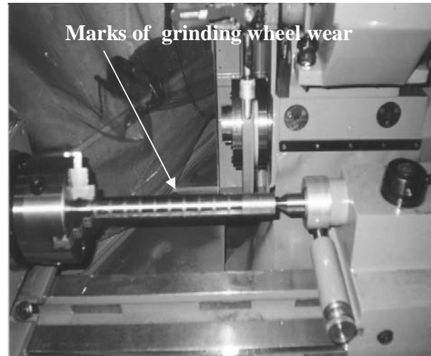
Figure 2. Grinding wheel diametral wear measurement.
