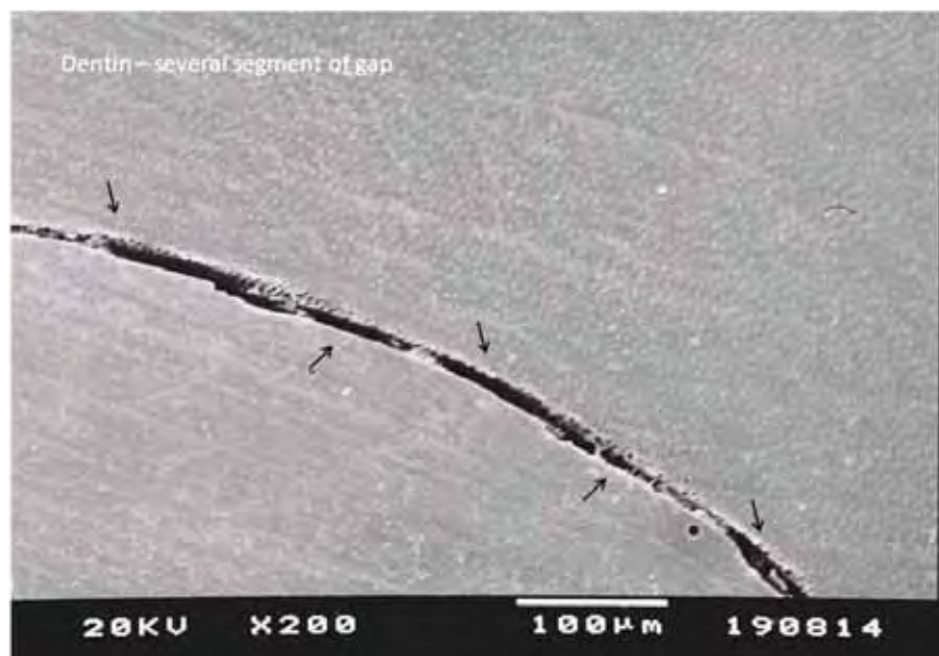
Fig 3 – Representative image of the external adaptation after thermal cycling.
