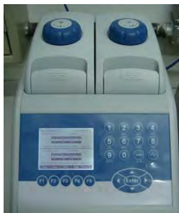
Figura 21 – Termocicladora Gene Pro (Thermal Cycler, BIOER Technology Hangzhou, China).
