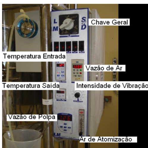
Figura 3.15: Painel de controle do spray dryer .
