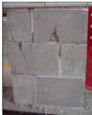
$\frac{1}{4}$  Par B1 AI1
