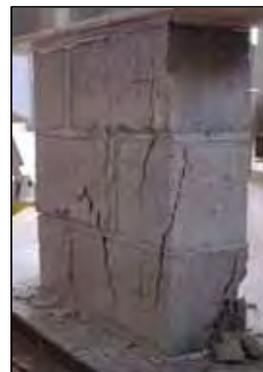
$\frac{1}{4}$  Par B1 AI2.**Figura 4.13 – Forma rompida das  $\frac{1}{4}$  Par.**
