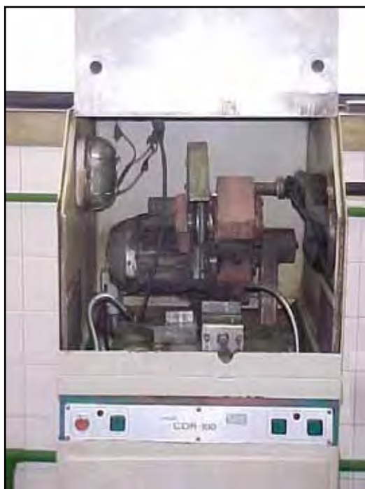
Figura 42 – Máquina “Cut-off” (Gentileza Tenaris Confab)
