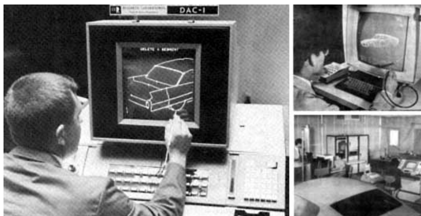
Figura 18 – DAC-1 da General Motors: Computer Aided Design (1964).
