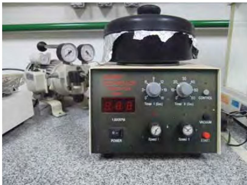
Figura 8 – Spin Coater , Model KW4, Chemat Technology INC
