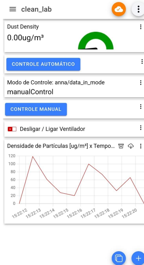
Figura 9 - Interface do painel de controle elaborado no IoT MQTT Panel.
