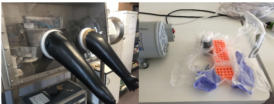
Figure A3 – Glove box (left) and glove bag (right) for AgNP storage procedure.
