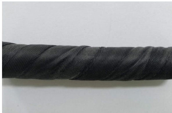
Figura 14 – Overlap de Fita de Bandagem
