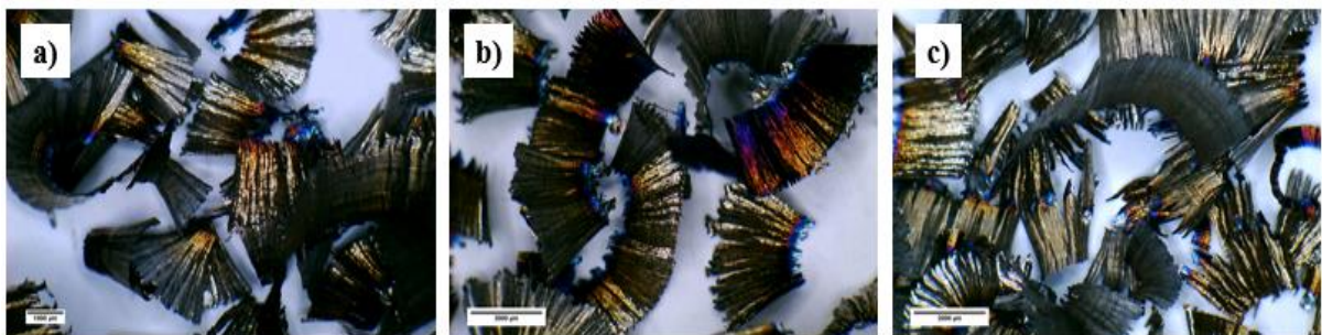
Figure 102 – Variation of the chip form to f of 0.10 mm/rev, using the \text{Al}_2\text{O}_3 -MgO ceramic cutting tools (0.80x). a) v_c of 700 m/min; b) v_c of 800 m/min; c) v_c of 900 m/min.
