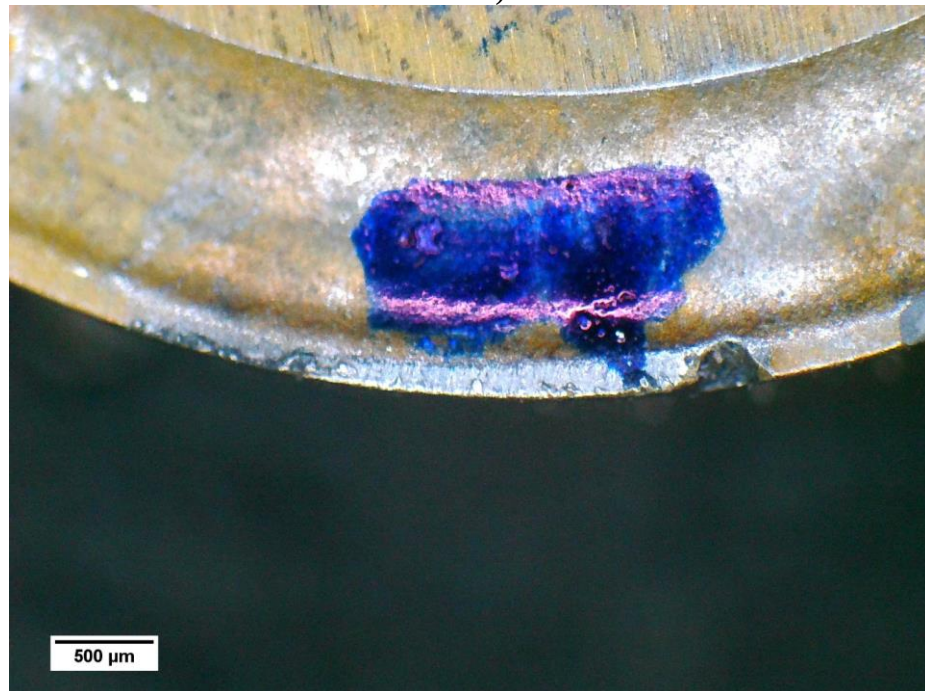
Figure 69 – Notch wear to the coated carbide tools rake face ( v_c of 100m/min and f of 0.10 mm/t).
