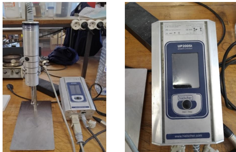
Figure 10 - Ultrasonic processor for the particle's dispersion in the electrolyte.
