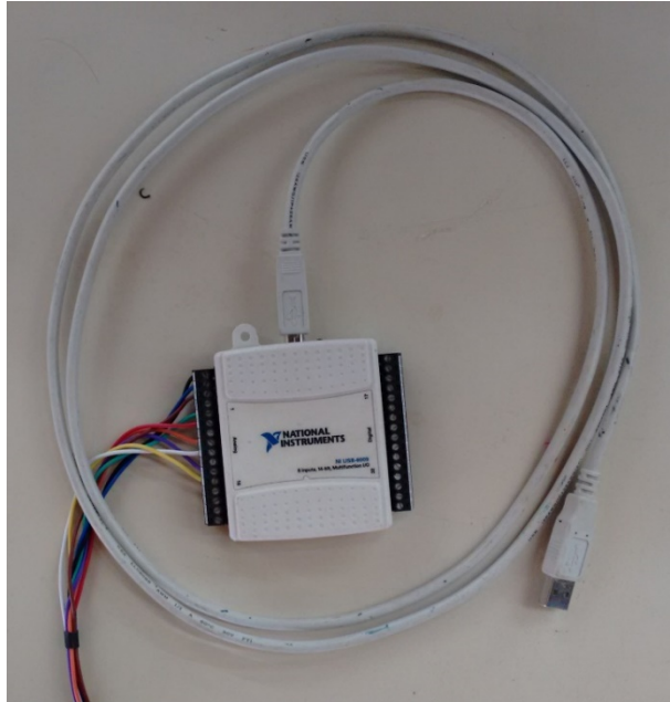
Figura 11 - DAQ NI USB-6009 da National Instruments .
