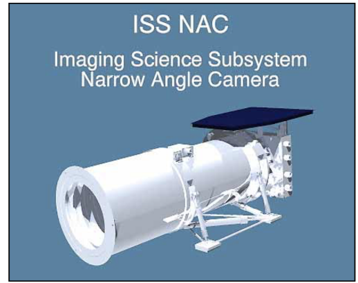
Figure 6.1: The Imaging Science Subsystem of Cassini Spacecraft (ISS) (left), and The Imaging Science Subsystem Narrow Camera (ISS NAC) (right); The ISS consisted of a wide-angle and a narrow-angle digital camera. The narrow-angle camera provided high resolution images of, among other, the surfaces of Saturn’s moons.
