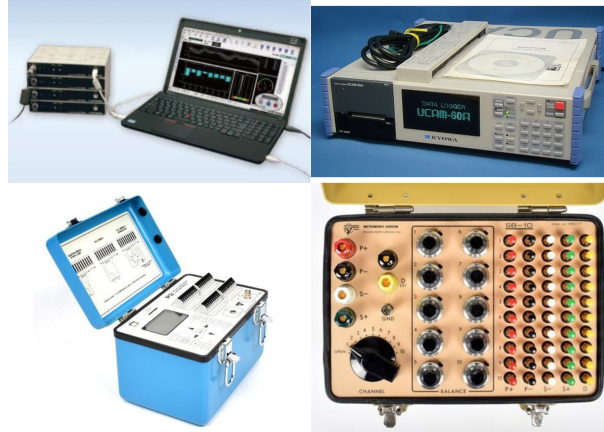
Figure 7. Conventional strain gauge data logger systems
