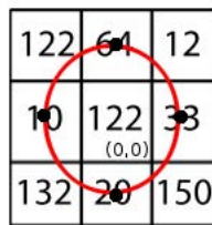
Figure 13 – Example of a LBP_{(4,1)} neighborhood of a pixel. The black dots are the sampling points in the red circle.
