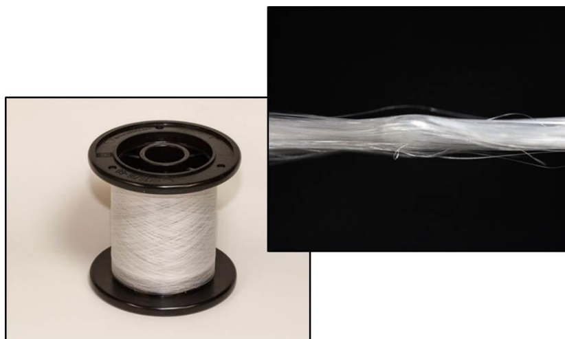
Figura 4. Biosteel Spidersilk Fibers produzida pela AMSilk® high performance materials.
