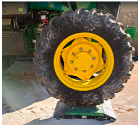
Figure 2. Obtaining tractor weight using pad scales.
