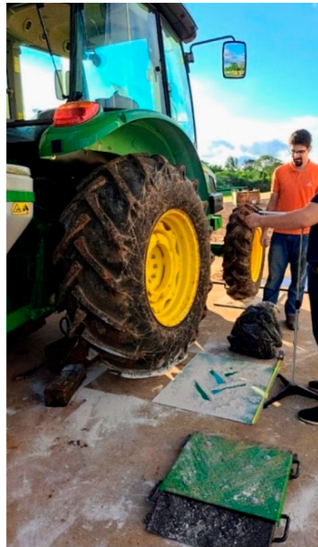
Figure 3. Tire contact area collection. The person shown in this figure is the first author of the manuscript.
