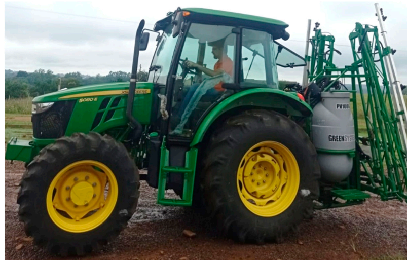
Figure 1. John Deere 5080E tractor coupled to Greensystem PV1006 sprayer used in the experiment. The person shown in this figure is the first author of the manuscript.
