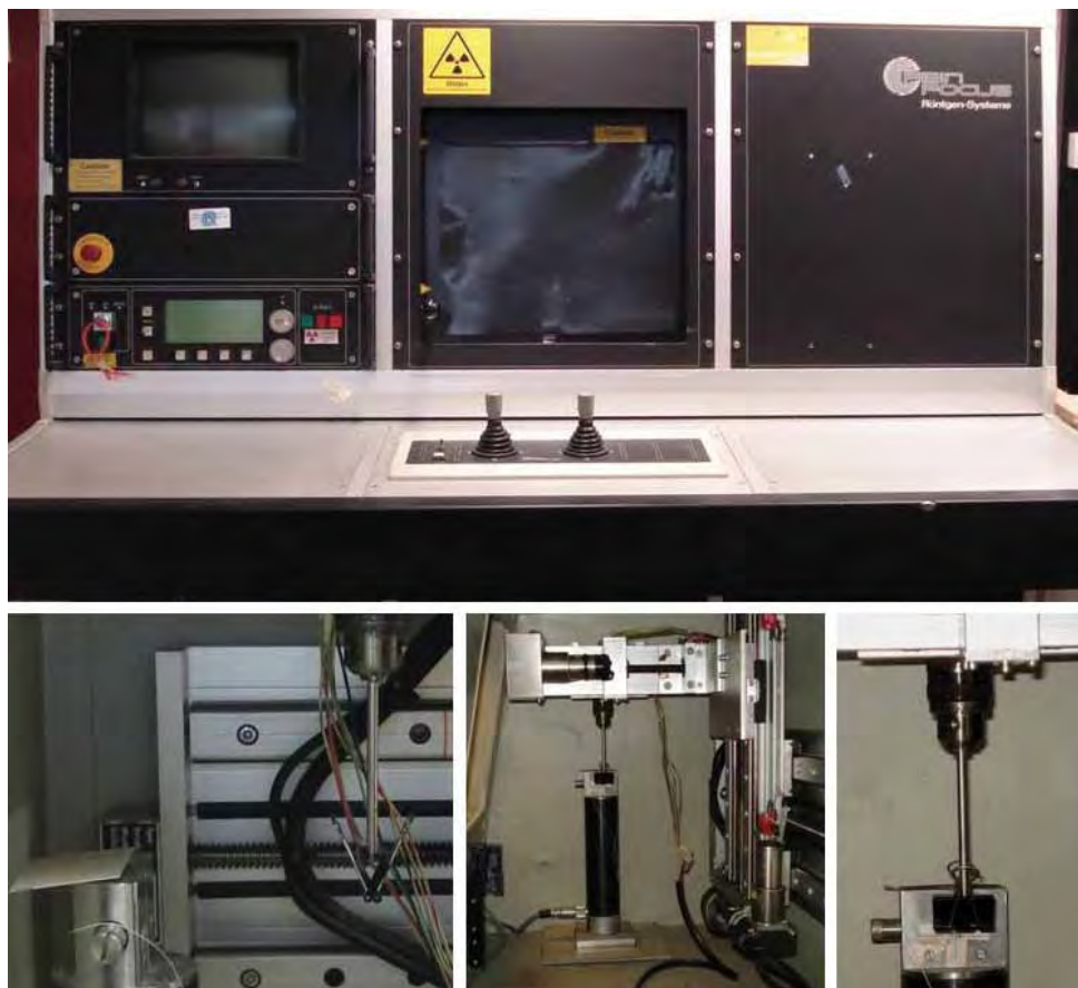
FIGURA 12 - RADIOGRAFIA DIGITAL - IMAGE PLATE: IPX (GE IT) TUBO DE RAIOS X: FXS-100.10 (FEINFOCUS).
