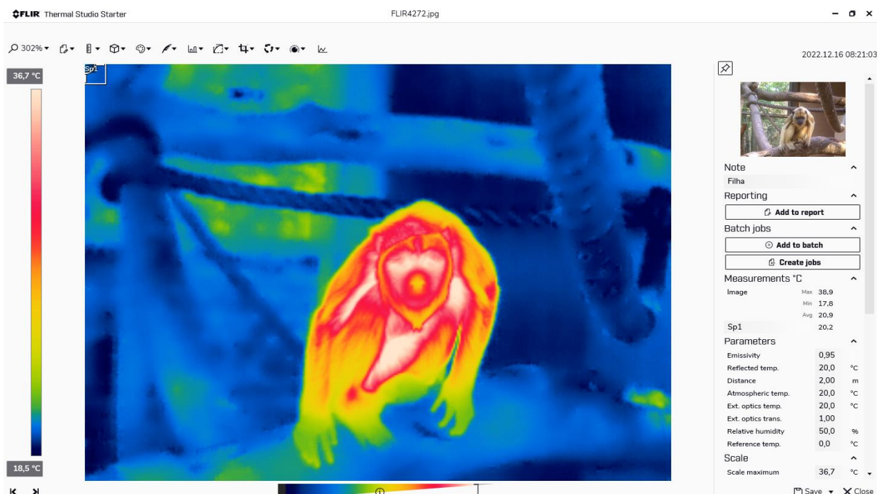
FIGURE 1 – Thermographic image of a black-and-gold howler monkey in the software. It is possible to compare the animal colors with the standardized colors in the Rainbow pattern multicolor bar on the left of the photo. In this established standard, dark blue represents lower temperatures (18.5°C) and white represents higher temperatures (36.7°C). Photo: André L.M. Costa.
