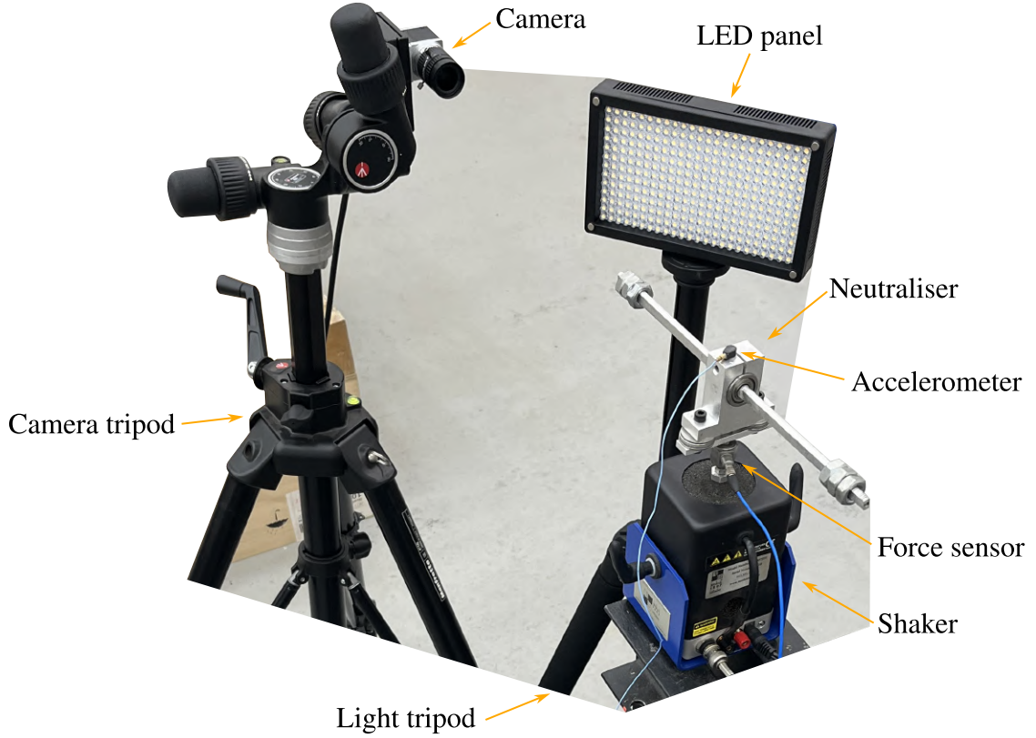
Figure 4.2: The rig used for the harmonic excitation. The neutraliser is attached to the shaker through a force sensor and has an accelerometer on the base. The high-speed camera and the light source are positioned to record the rotation of the neutraliser.
