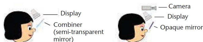
Figura 8 - Comparativo entre 'optical see-through' e 'video see-through'
