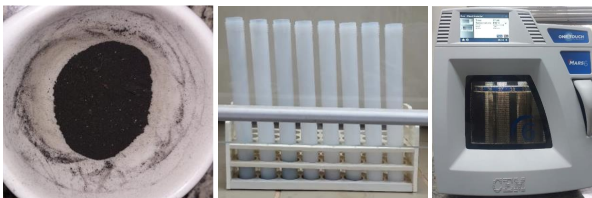
Figure 2. From left to right: Finely ground charcoal ready for analysis; Tube containing the sample and digestive reagents; Tubes in the microwave.
