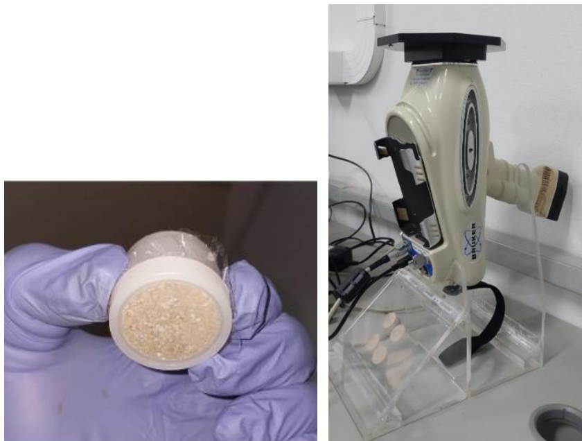
Figure 4. Ground sample pressed into the sample holder and BRUKER C3 portable X-ray device
