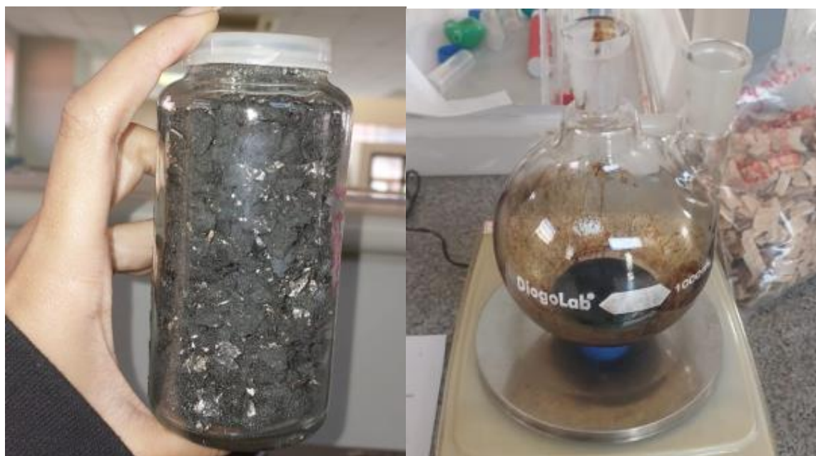
Figure 5. From left to right: charcoal and pyroligneous liquor obtained from the carbonization process of the residue from used beverage carton recycling
