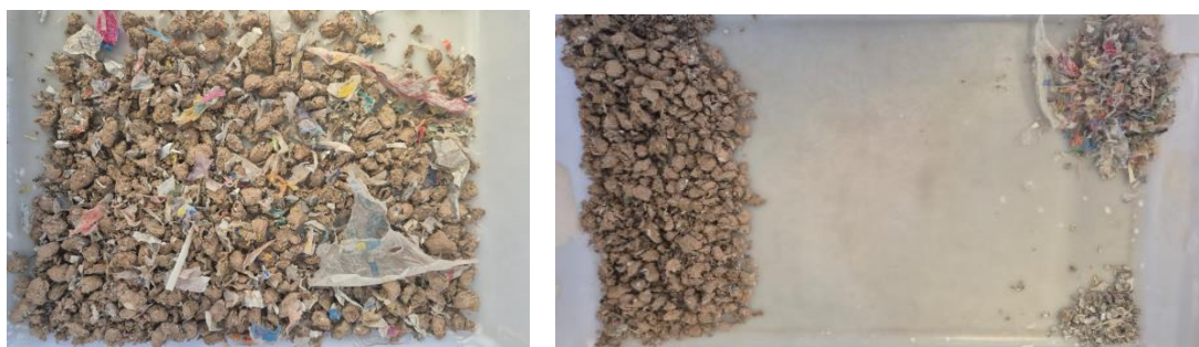
Figure 5. From left to right: Residue before separation and residue after separation with its components: Paper and Plastic + Aluminium.
