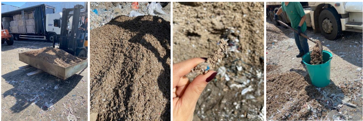
Figure 2. Residue collected at the PolyAl Recycler's site – the image shows (from left to right) the residue exiting the centrifugation process, the stored residue pile, a close-up of the residue, and the residue being stored in a bucket for laboratory analysis
