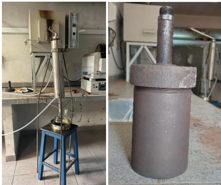
Figure 1. From left to right: A) Laboratory muffle coupled to the system of glass condensers and volumetric flask, used during the pyrolysis and collection of pyrolytic liquors; B) Metallic container.
