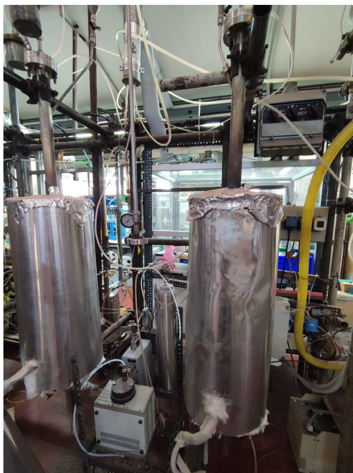
Figure 25 – Photo of the DIFB system in operation at University of Naples
