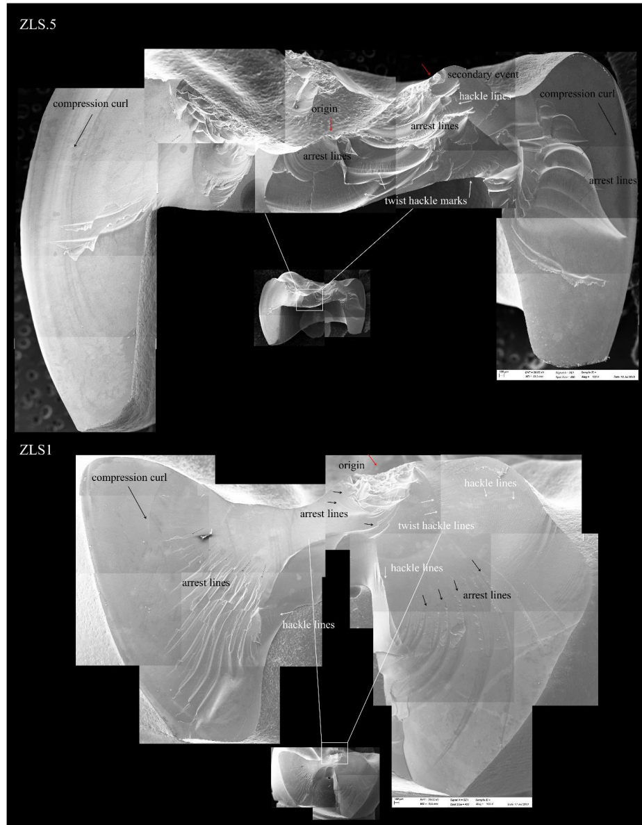
Figure 6. Fractographic analysis of representative ZLS 0.5 and 1 mm crowns. Compression curl, twist hackle marks, arrest and hackle lines determined that the crack started on the occlusal surface and propagated through to the bottom of the restoration. The ZLS crowns showed many arrest lines which indicate the failure origin. However, the damage accumulation in fatigue experiments could generate events other than the origin, i.e. secondary event(s). The specimens were evaluated under 40x and 100x magnifications.
