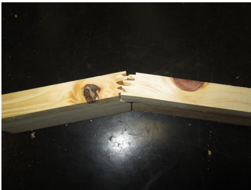
Figura 36: Ruptura na emenda de finger joint , painel classe C.
