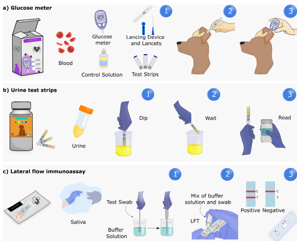
Figure 11. Schematic representation of common commercial POCTs for pet diagnostics and health monitoring. (a) Pet blood glucose monitoring: (1, 2) blood collection using a lancing device and (3) glucose detection. (b) Test strips for urine analysis: (1) immersion of the sensor strip in urine, (2) reaction between the analyte and receptors within the device, and (3) color change based on the analyte concentration. (c) LFT for detecting biomarkers in animal saliva: (1) saliva collection using a test swab, (2) addition of the sample dilution in buffer and addition to the LFT device, and (3) results displayed on the device after the incubation period.
