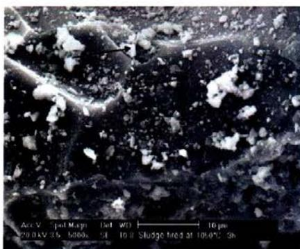
Fig. 2 Typical SEM image of sintered sludge fired at  $1050^\circ\text{C}$  (5000 $\times$ )
