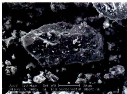
Fig. 1 Typical SEM image of sintered sludge fired at  $1050^\circ\text{C}$  (2000 $\times$ )
