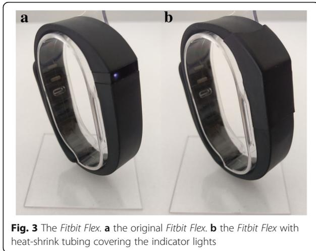
**Fig. 3** The *Fitbit Flex*. **a** the original *Fitbit Flex*. **b** the *Fitbit Flex* with heat-shrink tubing covering the indicator lights
