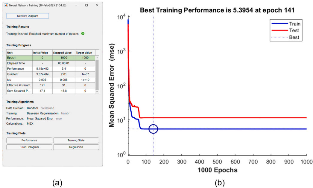
Fig. 2. Training parameters (a) and performance (b) of an ANN in MATLAB 2024b.
