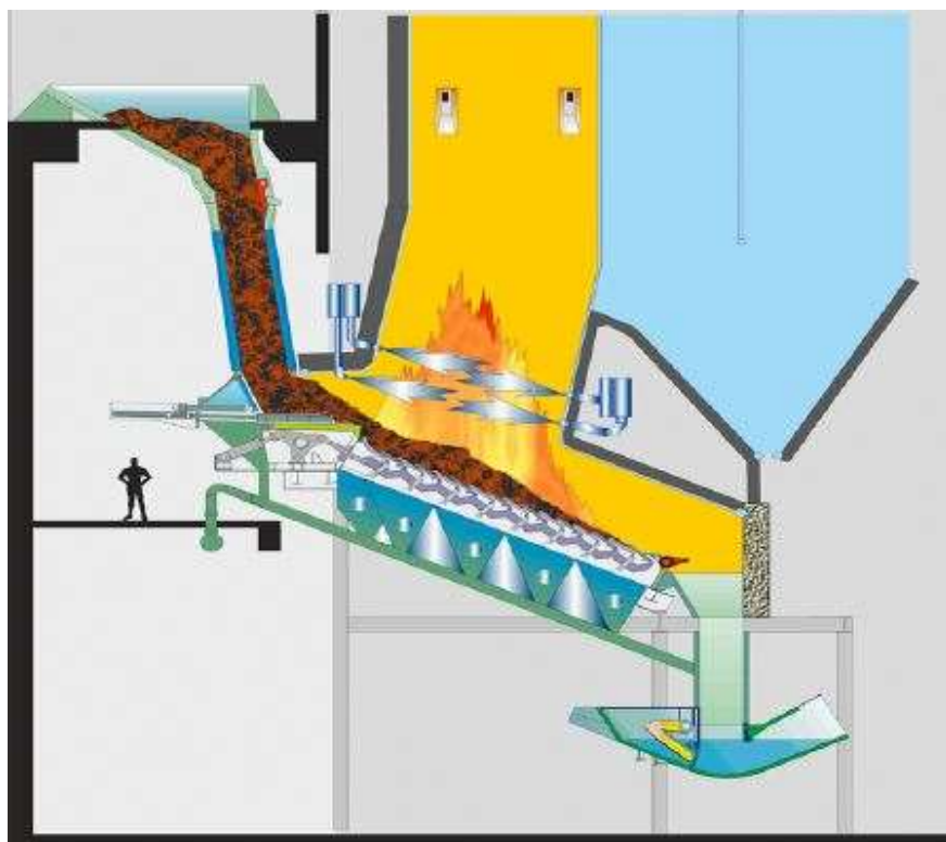
Figura 19 - Esquema de Câmara de Combustão; Fonte: Guidebook for the application of waste to energy Technologies in Latin America and other developing regions
