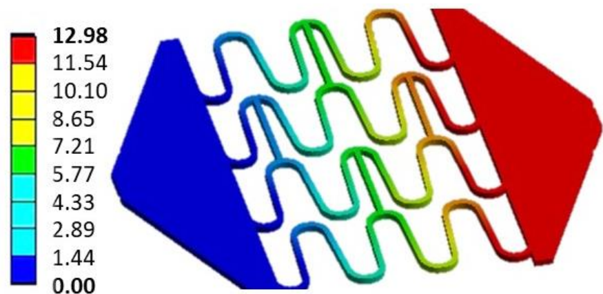
Figure 7. Finite element simulation of customized 3D-printed PLA stent specimens. Displacement in millimetres.
