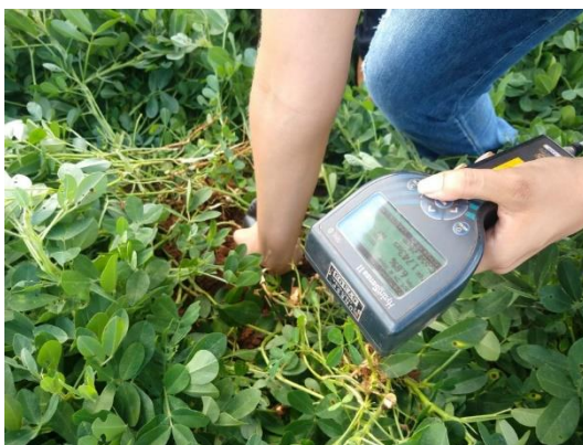
Figura 4. Sonda TDR (Time Domain Reflectometer).
