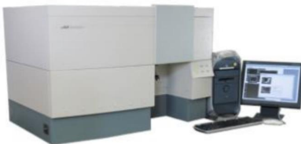
Figura 2: Becton Dickinson (BD) FACSCalibur Flow Cytometer 4 Color.
