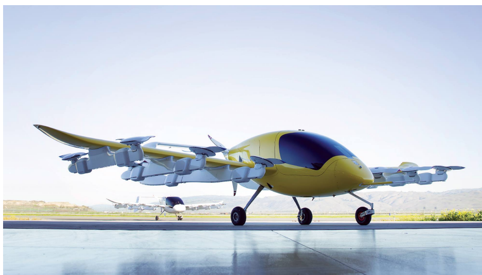
Figura 5 – Modelo de eVTOL Lift + Cruise Wisk Aero Cora (Generation 5)
