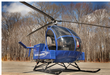
Figura 8 – Modelo de eVTOL Electric Rotorcraft Sikorsky Firefly
