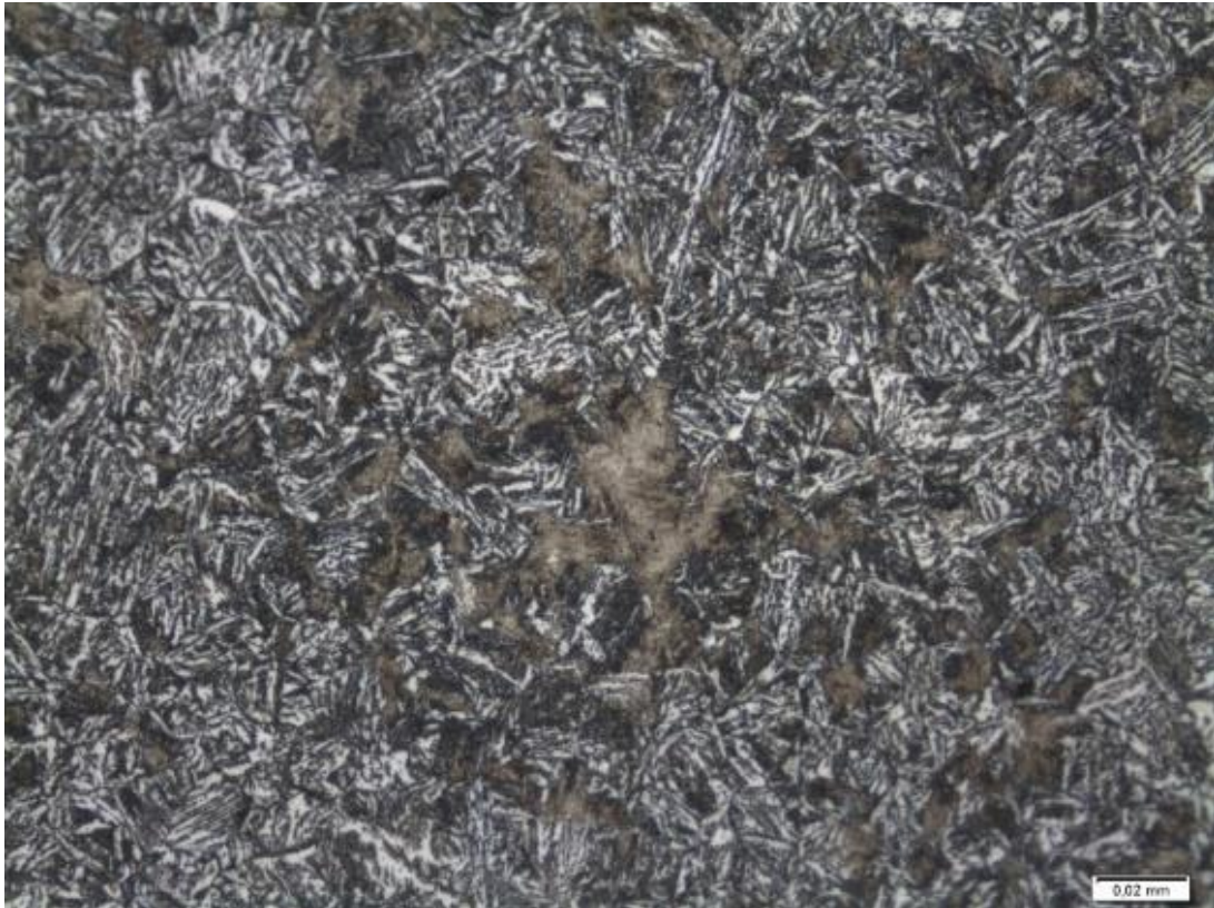
Figura 12: Amostra 2, Bloco, 50% Bainita, 26% Ferrita, 14% Martensita, 375HB.
