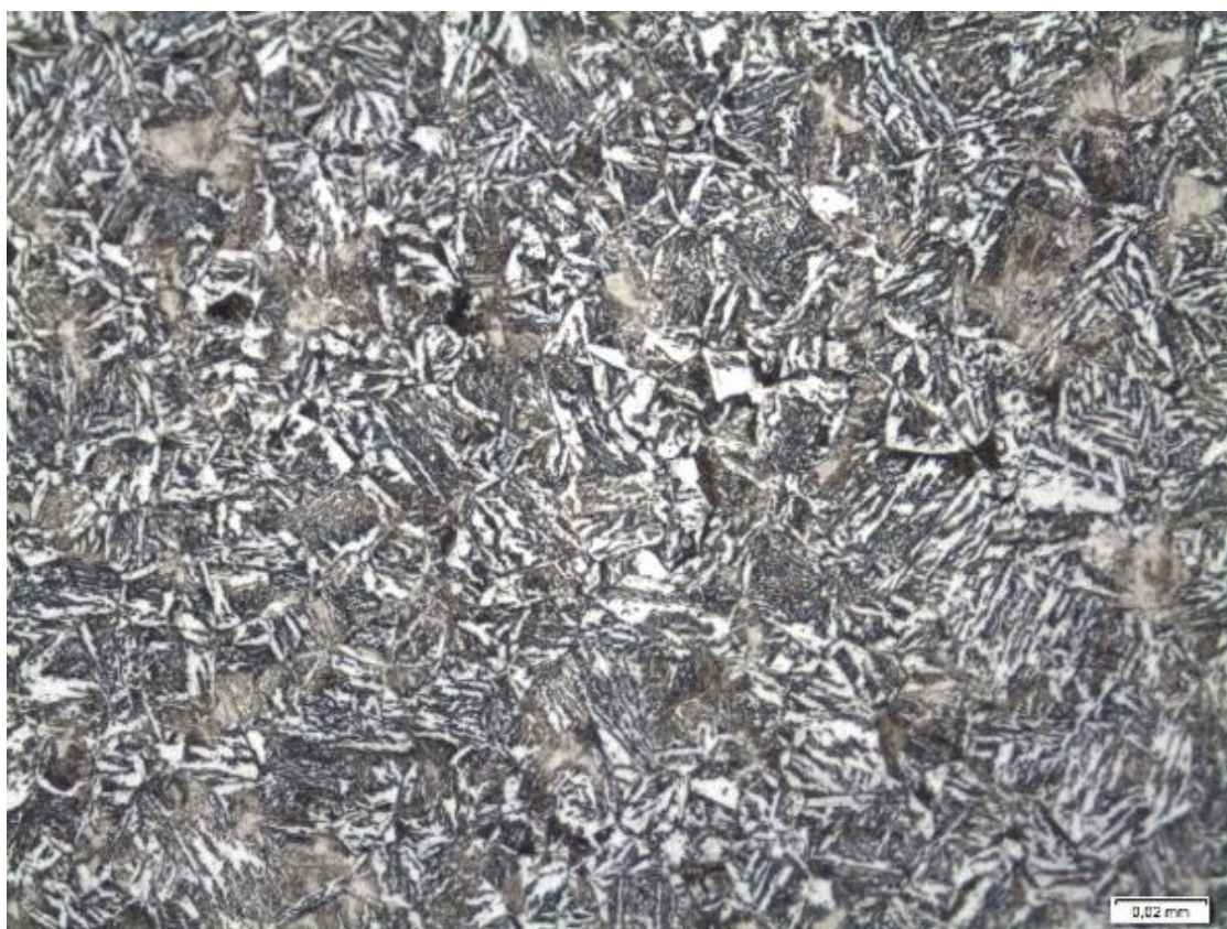
Figura 11: Amostra 1, Bloco, 63% Bainita, 21% Ferrita, 16%Perlita, 352HB.
