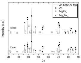
Figure 4. Patterns of X-ray diffraction.
