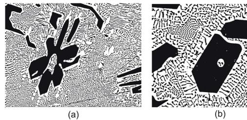
Figure 12. Binary images (using the ImageJ® software): (a) sample P\_10mm IMCs = 39% and (b) sample P\_70mm IMCs = 50%.
