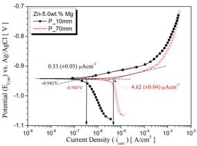
**Figure 10.** Potentiodynamic polarization curves of the Zn-5.0wt.%Mg alloy for samples of positions P\_10mm and P\_70mm.
