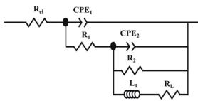
**Figure 9.** Schematic representation of the equivalent circuit (EC) used for P\_10mm and P\_70mm.
