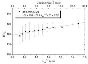
**Figure 7.** Vickers microhardness profile ( $HV_{0.5}$ ) as a function of the eutectic interphase spacing ( $\lambda_{eur}$ ) and cooling rate ( $\dot{T}$ ).
