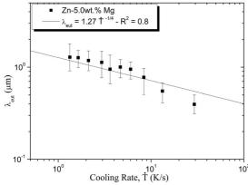
**Figure 6.** Evolution of the eutectic interphase spacing  $(\lambda_{eut})$  as a function of the solidification cooling rate (T).
