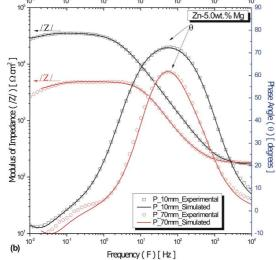
**Figure 8.** Comparison of the experimental and simulated CNLS results for the Zn-5.0wt.%Mg alloy samples P\_10mm and P\_70mm: (a) Nyquist graphs; High frequencies values indicated at the semicircles are related to the maximum imaginary component; while low frequencies values are related to the start of the inductive behavior. (b) Bode and Bode-phase graphs; The arrows indicate the maximum angle (θ) and the impedance module (/Z/) values.
