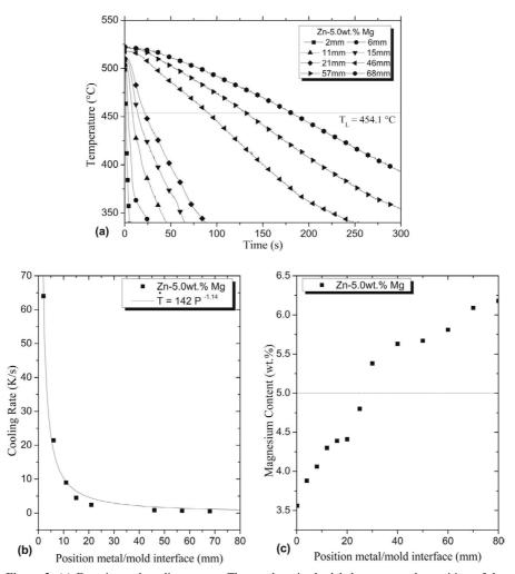
**Figure 2.** (a) Experimental cooling curves; The numbers in the label, represent the position of the thermocouples (P) from the cooled bottom of the casting (P=0); (b) Cooling rate as a function of (P); (c) Mg concentration profile along the length of the vertical DS casting.
