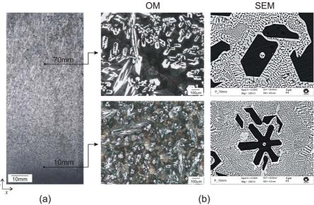
**Figure 3.** (a) Macrostructure and (b) Microstructure in optical microscope (OM) and scanning electron microscope (SEM) for positions: P\_10mm and P\_70mm, in which P is the distance from the cooling bottom.
