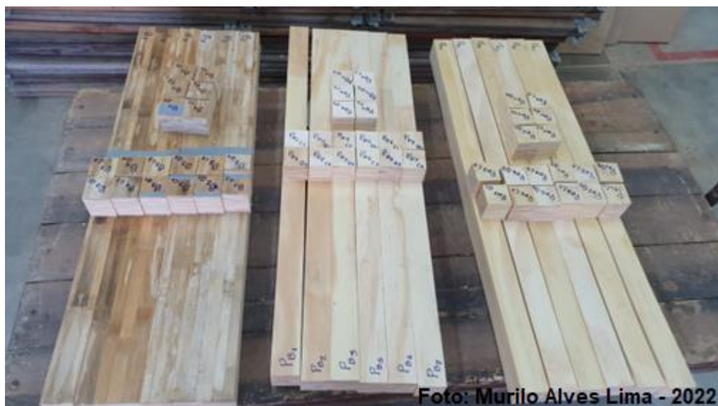
Figura 14 – Corpos de Prova do Laminated Veneer Lumber
