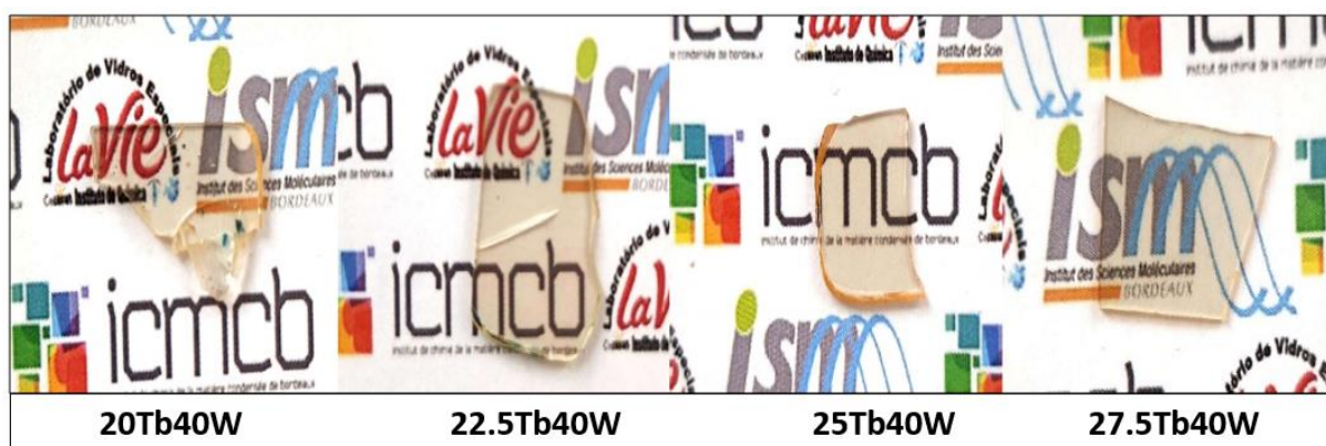
Figure 19. Samples xTb_2O_3 - (60-x)B_2O_3 - 40WO_3 series, after cut and polishing, with their specific names. (Own authorship).
