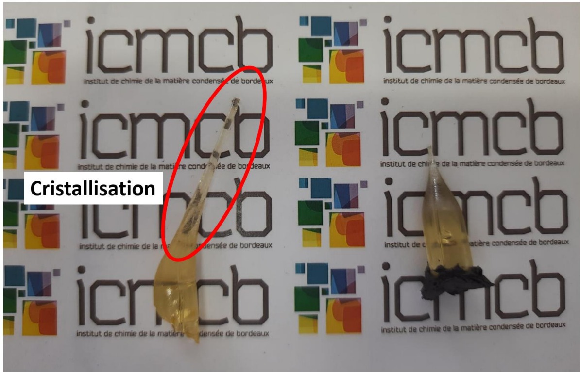
Figure A-2. Preforms after trying to draw the fibers. A crystalline phase is observed in the region where preform heating occurred.
