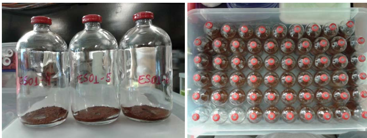
Figure 6. Process of incubation in which triplicates consisting of soil and deionized water were placed in vials and sealed with butyl rubber septa.
