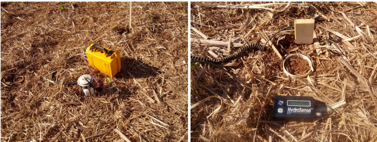
Figure 4. Portable LI-8100 system (on the left) used to measure the in situ soil CO 2 emission and soil temperature, and TDR system (on the right) used to measure the soil moisture in the experimental area.
