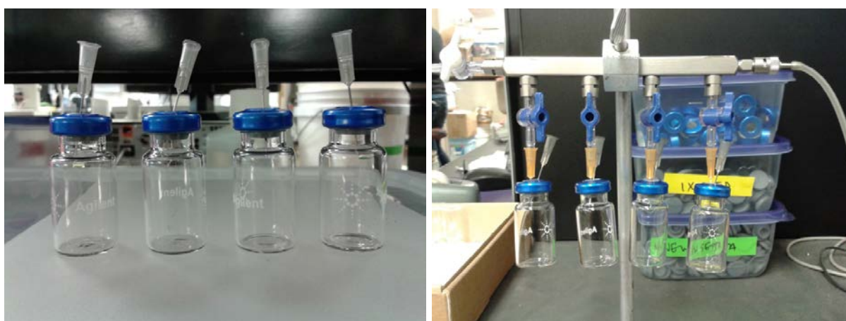
Figure 7. Process of flushing helium into vials used to analyze the headspace gas samples in the gas chromatograph.
