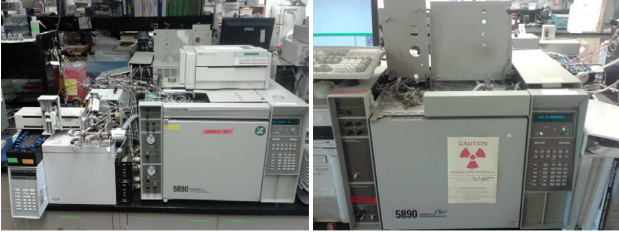
Figure 8. Gas chromatograph with three different analytical columns used to assess the production rate of soil greenhouse gases.
