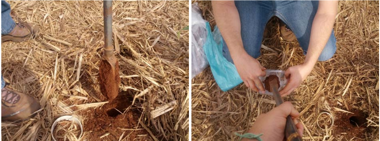
Figure 5. Extraction of soil samples from a depth of 0–10 cm from all 133 grid points in the experimental area.
