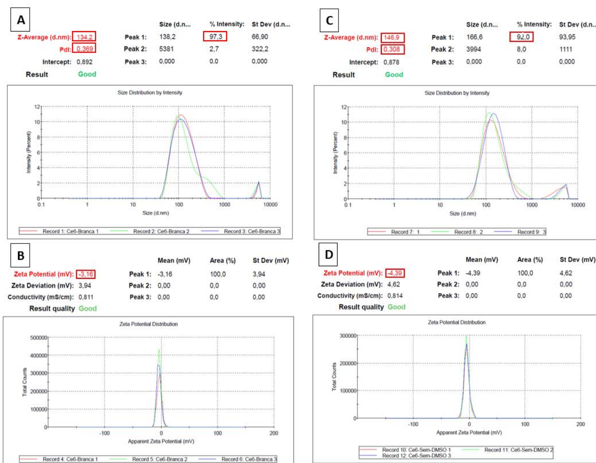
Figure 1: Droplet size, polydispersity index and zeta potential of nanoemulsion (A e B) and Ce6-loaded nanoemulsion (C e D).
