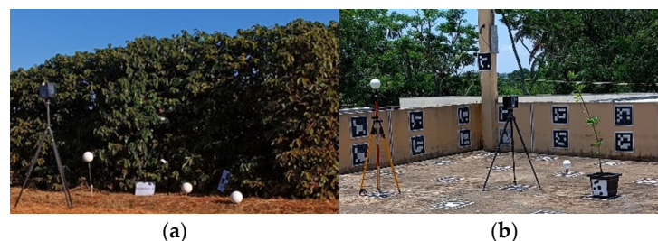
Figure 2. (a) Coffee plantation with targets and spheres. (b) Experimental setup with ARUCO markers on the floor and walls, and a potted apple tree.
