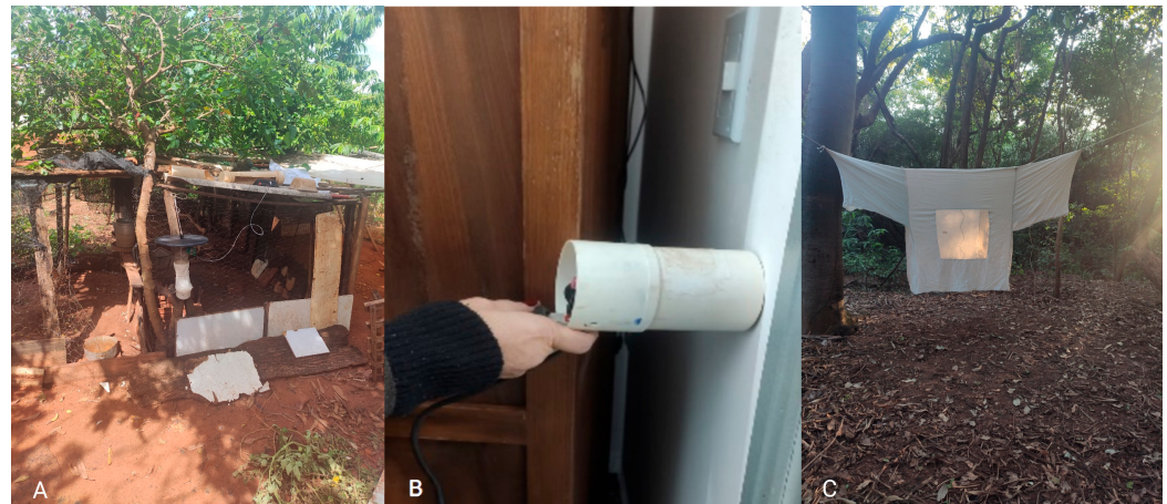
Figure 2. Capture methodologies: (A) CDC light traps; (B) manual capture using electric aspirators; and (C) Shannon tent trap.
