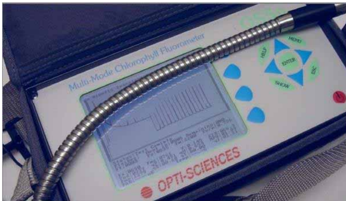
Figura 2 Painel frontal do fluorômetro portátil OS5p. Botucatu/SP, 2015.
