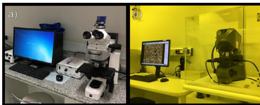
Figure 18: Instruments used for the optical microscopies performed in this work. (a) Conventional optical microscope Zeiss Axio Imager. (b) LSCM from Keyence VK-X200. Source: Images acquired and adapted from the official LNNano site 1 , at 18/03/2023.
