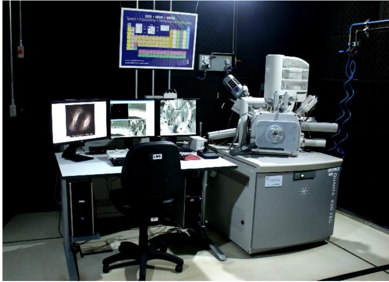
Figure 20: Scanning Electron Microscope (FEG-SEM) Inspect F50 from FEI (Japan). Source: the author.
