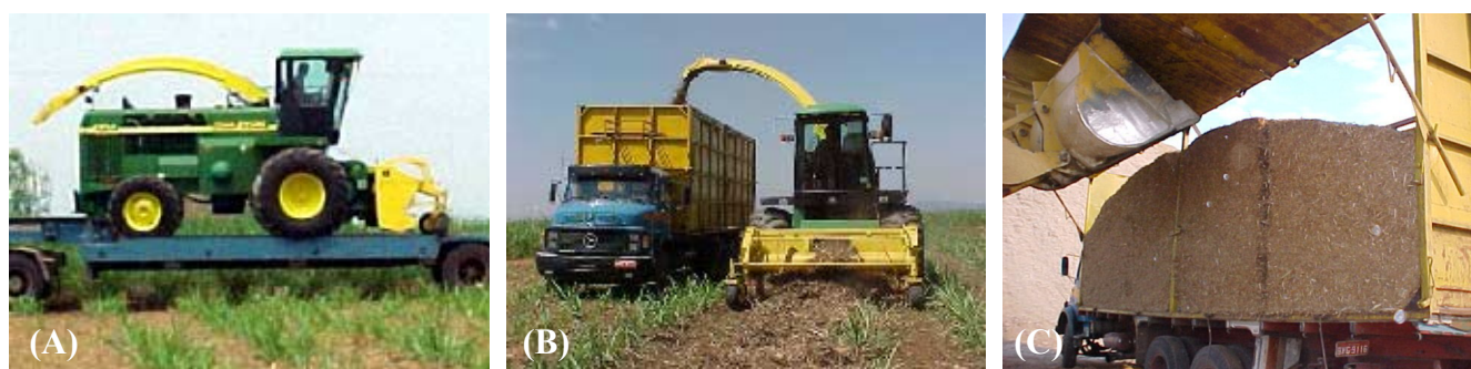
Figure 2 – Side view from de JOHN DEERE ® forage harvester (A), harvester in operation with the truck (B) and unloading proceeding of the residues in the mill (C).
